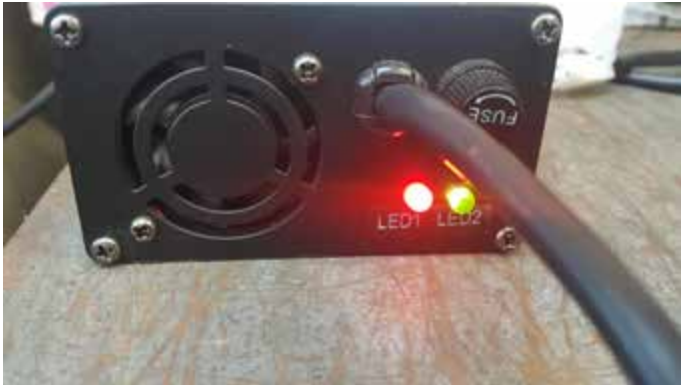
Figure 3. The charger supplied is a smart charger and indicates its status via two LEDs.
